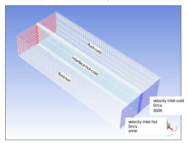
The "interface-hot-cold", which is a wall between the zones "fluid-hot" and "fluid-cold" was defined with the Shell Conduction Manager as displayed in the picture below
