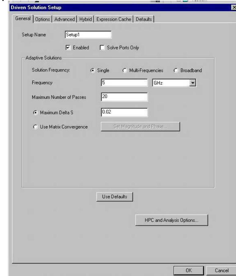
Since this array is intended to operate at 5GHz, we will set the solution frequency to 5 GHz. We will also change the maximum number of passes to 20.
