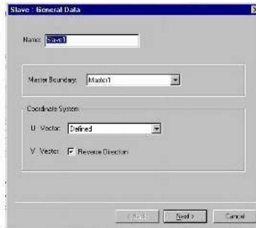
Define the U Vector along one of the edges of the slave face by clicking the corners corresponding to those you chose on the Master boundary, as shown below. If necessary, click the “reverse direction” option on the V vector, so that the U and V vectors frame the face, as shown below.
