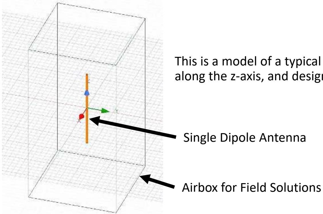
This is a model of a typical dipole antenna, oriented along the z-axis, and designed to operate at 5 GHz.
