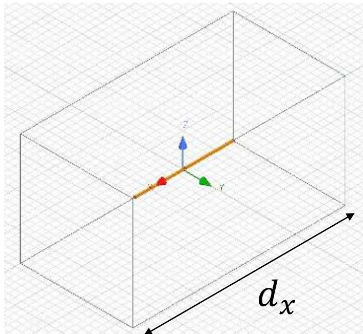
$$d_x = \lambda = \frac{3 \times 10^8 \text{ m/s}}{5 \times 10^9 \text{ Hz}} = 60 \text{ mm}$$
