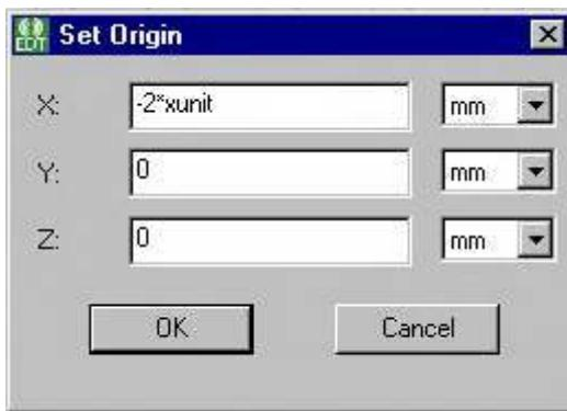
Hit the F4 button on your keyboard to toggle dialog input, then enter the distances by which you wish to shift the origin in order to center it along the array. In the case of our linear array along the x-axis, this only involves a shift in the negative x-direction, equal to twice the unit cell's x-dimension.
