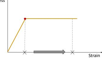
Strain jumps without any load increment
