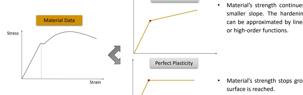
Material's strength continues to grow, but with smaller slope. The hardening part of plasticity can be approximated by linear, piece-wise linear
