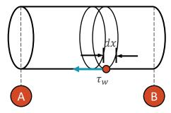
• We can analyze this flow following an approach like the one used for Rayleigh flow. However, this time we need to include the frictional effects in the momentum equation:
