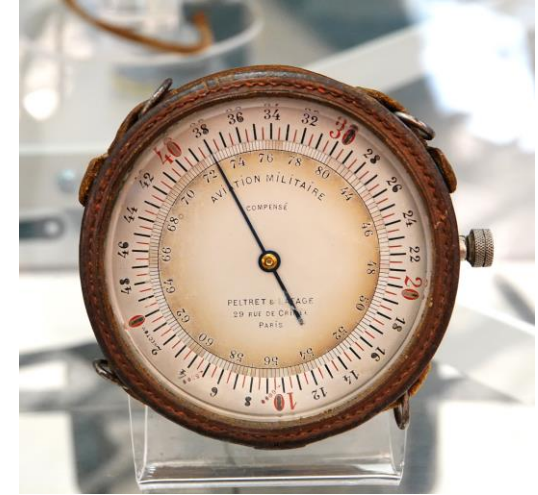
Pressure altimeter used for aircraft altitude
