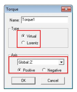
Note: if Virtual is selected, the system uses virtual work principles to compute the torque on an object
