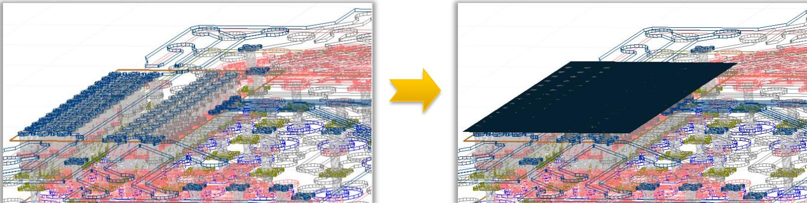
To create Flipchip bumps for the component, we define the Solder Ball properties to the FCHIP component. A reference plane for the Flipchip bumps is automatically added to the geometry.
