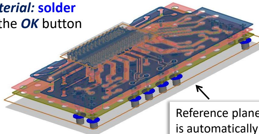
Reference plane for the BGA Solder Balls is automatically added to the geometry.
